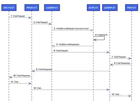
*Figure 32: Simplified message sequence (AT in AT)*
