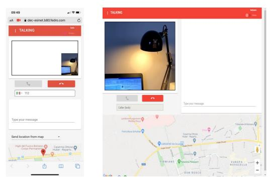
*Figure 38: webRTC client (left) and PSAP user interface, with ongoing videocall and location of the caller (blue icon in the center of the map)*
