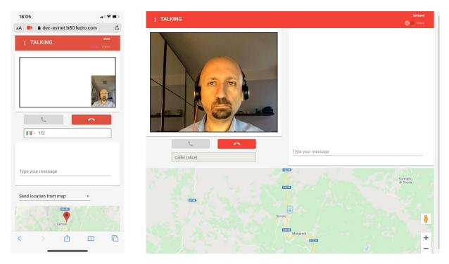
*Figure 55: webRTC client (left) and PSAP user interface, with ongoing videocall and location of the caller (blue icon in the center of the map). The location, Senale, is corresponding to 112 Bolzano PSAP in the NG112 call scenario.*
