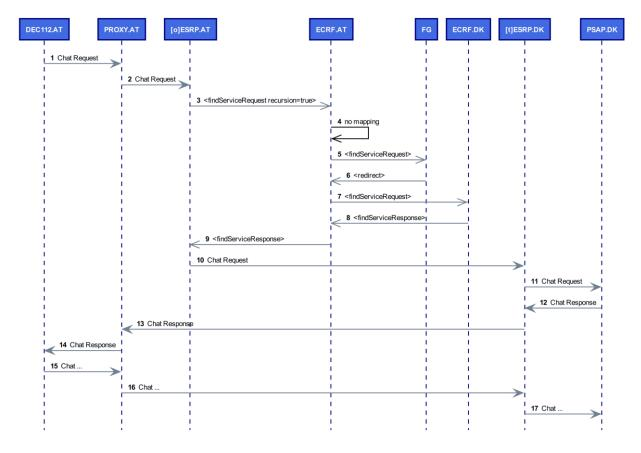
Figure 46: Simplified message sequence (AT in DK)
