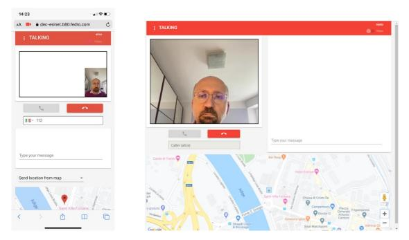
*Figure 41: webRTC client (left) and PSAP user interface, with ongoing videocall and location of the caller (blue icon in the center of the map)*
