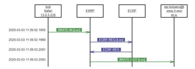
Figure 39: call chart, with time delays expressed on the left-hand side
