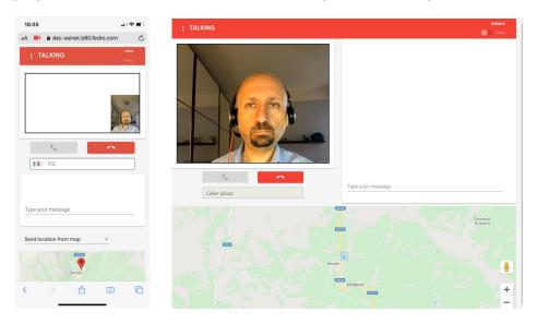
*Figure 6: webRTC client (left) and PSAP user interface, with ongoing videocall and location of the caller (blue icon in the center of the map). The location, Senale, is corresponding to 112 Bolzano PSAP in the NG112 call scenario.*
