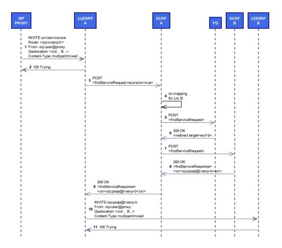
Figure 24: Multimedia conversation (initial setup message; roaming)
